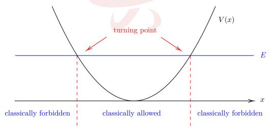
The WKB approximation scheme looks for solutions of the stationary wave function of the exponential form (notation clarification: S(x) here is not the S-matrix)
