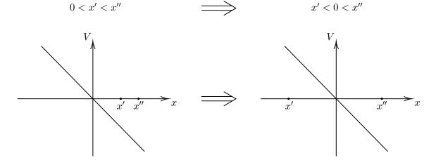
We would like to keep track of the semi-classical approximation along the deformation of x'. However, if we simply change x' along the real axis, we will soon run into trouble when x' hits the turning point 0. In fact when x' = 0, the velocity at the turning point vanishes
