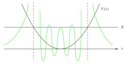
WKB approximated solution. Amplitude blows up near the turning points.
