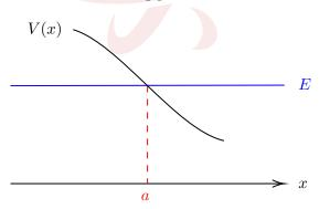
$$\frac{A}{\sqrt{\lambda(x)}} \exp\left(-\int_{x}^{a} \lambda(y) \, dy\right) \qquad \Longrightarrow \qquad \frac{2A}{\sqrt{k(x)}} \cos\left(\int_{a}^{x} k(y) \, dy - \frac{\pi}{4}\right)$$
