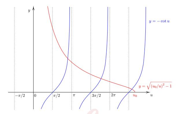
Again, we find only finite number of intersections. The number of odd bound state is bigger for larger  $u_0$ , i.e., for wider and deeper well. However, for  $u_0$  sufficiently small, say  $u_0 < \pi/2$ , there will be no odd bound state.
