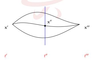
Thinking about  $K(\mathbf{x}''', t'''; \mathbf{x}', t')$  as a transition amplitude from  $\mathbf{x}'$  at time t' to  $\mathbf{x}'''$  at time t''', the composition law says that this transition amplitude is the same as summing over all the transitions at the intermediate time t'' for all possible  $\mathbf{x}''$ .
