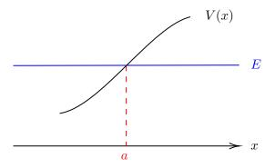
$$\frac{2A}{\sqrt{k(x)}}\cos\left(\int_{x}^{a}k(y)\,dy - \frac{\pi}{4}\right) \iff \frac{A}{\sqrt{\lambda(x)}}\exp\left(-\int_{a}^{x}\lambda(y)\,dy\right)$$
