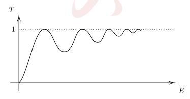
Note that there are certain values of E making T=1. In this case we have the full transmission as no waves are reflected: the well becomes transparent! From the above formula of T, the full transmission happens when
